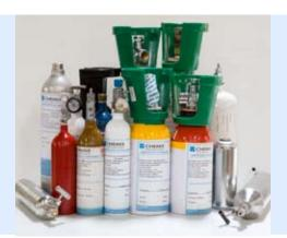
Calibration Gas Mixture- more emphatically a degree of measurement- is our prime product. Gravimetric filling method as per ISO 6142 where the components are added sequentially using traceable weights and improvised manometer method as per ISO 6146 are followed. For analysis, various GC methods and direct analysis methods as per IS, ISO and ASTM standards are used in the laboratory. Laboratory is maintained as per ISO 17025 (NABL). For certification, ISO 6141-2015 is being followed.
